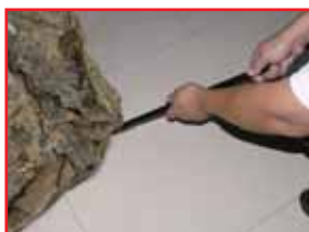
Medium-steel bar for prying, cutting, and digging work
